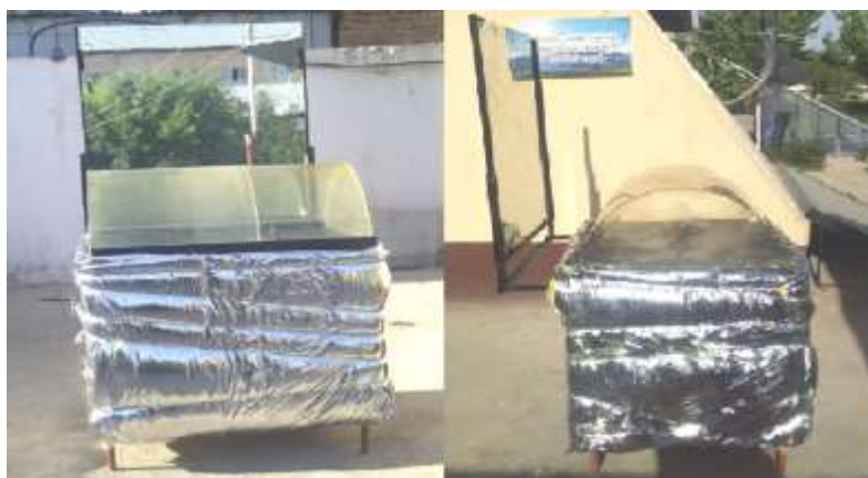
Fig.7. Experimental solar installation for the thermal processing of municipal solid waste
