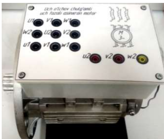
Fig. 2. Three-phase asynchronous electric motor with three measuring windings
